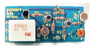
This project will let you make a switch that will be activated by light falling on a sensor. It is a very useful device and can be used in automatism's, security systems, counters, remote controls etc. It is very sensitive, fast acting and reliable. The circuit uses a Light Dependent Resistor (LDR) as a sensor and three transistors to amplify the signals from the LDR and drive the relay which does the switching.
